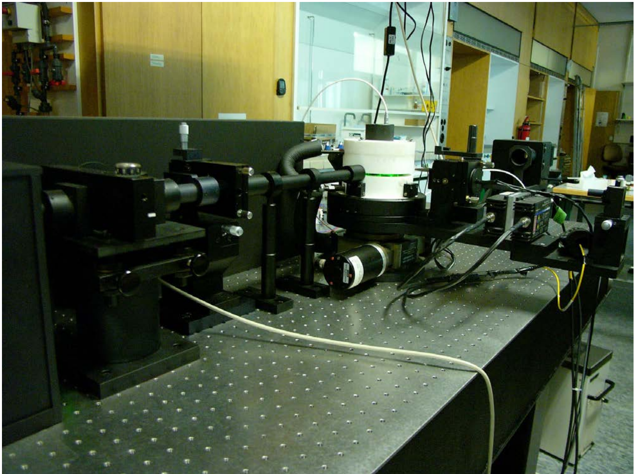
ALV/DLS/SLS-5000F monomode fiber compact goniometer system with ALV-5000 fast correlator
